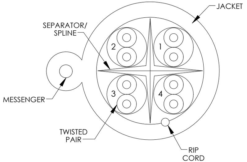
CAT6 550MHz, UTP, OUTDOOR RATED CABLE WITH MESSENGER, 4 TWISTED PAIR 23AWG SOLID-BARE COPPER
